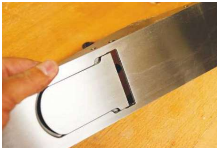
▲ The mouth is set into the sole, preventing any dig ins
